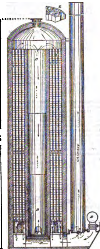
FIG. 11.—Diagram of Cowper Hot-Blast Stove at Duquesne. (After J. Kennedy.) Broken arrows show the path of the gas and air while the stove is "on gas," and solid arrows that of the blast while it is "on wind."
