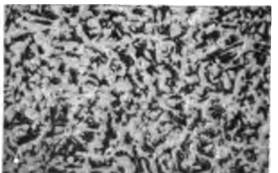
FIG. 6.—Gun steel, C. = 0.30%. From bottom of ingot as cast, magnified 29 diameters. Whites, ferrite; blacks, carbide.
