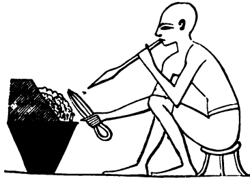
Egyptian Blowpipe, and small fireplace with cheeks to confine and reflect the heat. (Wilkinson.)
